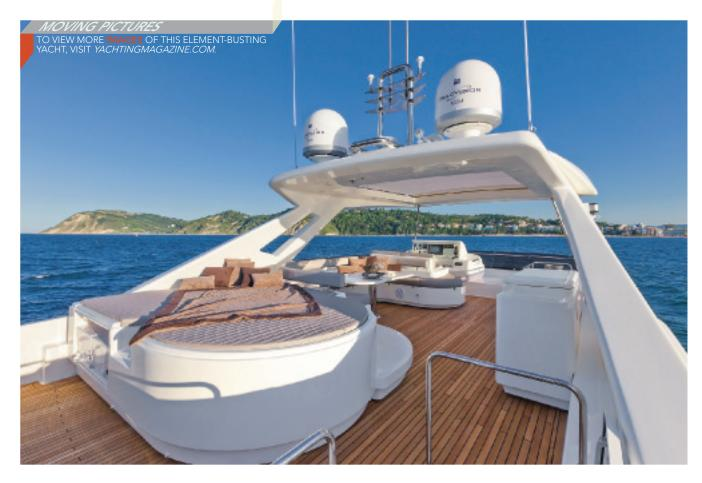
table and seating with a barbecue counter on the starboard side. Here there is a double grill, ice maker and fridge, which makes the spot a great open-air living area. Ferretti offers an optional fixed Bimini with an opening center to provide sun shelter. At the forward end, there is a reverse-angle windscreen that gives some wind shelter at the portside helm.
